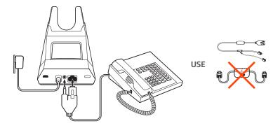
**IMPORTANT** Use configuration **A** on the bottom of the base, which works for most phones including Cisco phones.
