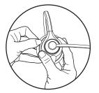
Once the bracket is in place, carefully feed the leatherette ear cushion over the bracket.
